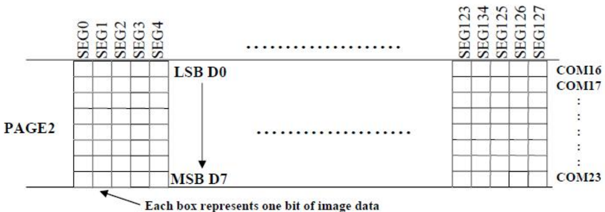
Figure 8-14 : Enlargement of GDDRAM (No row re-mapping and column-remapping)
